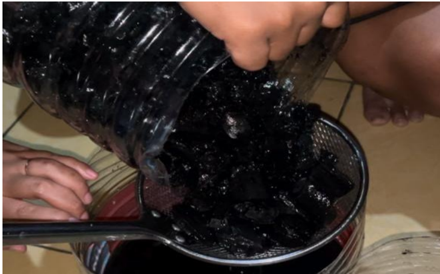
Figure 1. Used Cooking Oil Filtration Process
