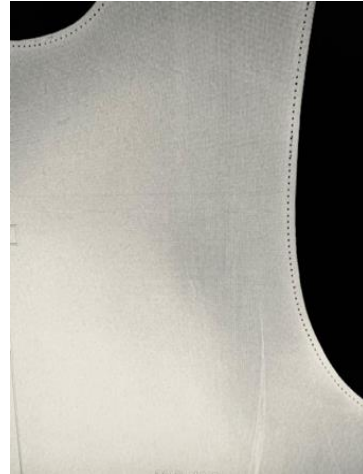
Gambar 8. hasil pengujian lead apron 2 kuadran 2. (RSUD Caruban, 2024)
