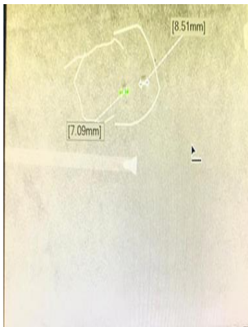
Gambar 9. Hasil pengujian lead apron 2 Kuadran 3. (RSUD Caruban, 2024)
