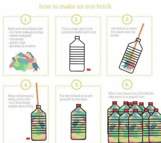
**Gambar 3.** Tahap pembuatan ecobrick ([Ecobricks — Zerowaste.id](https://www.ecobricks.com/))
